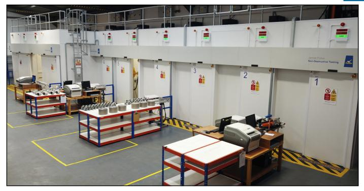
James Fisher NDT (JF NDT) offers extensive conventional and filmless Radiographic Inspection Services specialising in the radiography of safety critical components from a wide range of industry sectors including Aerospace and Automotive.
